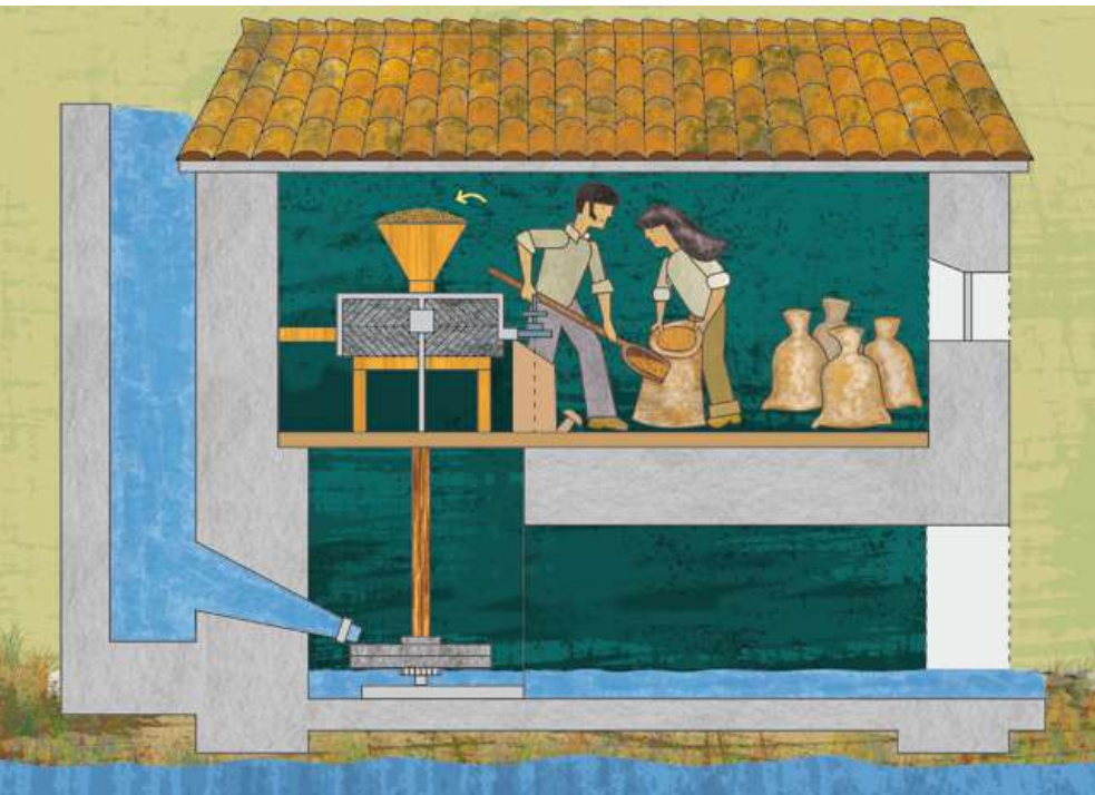
Diagram showing the functioning and the different parts of a hydraulic mill with a horizontal wheel.
